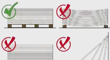
Resistant boards should be stored flat, raised from the ground on a pallet, in dry conditions indoors and be under cover. Boards should not be leaned upright for long periods of time
