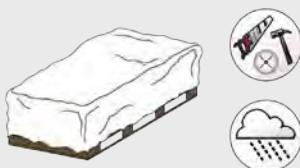
Any moisture allowed to infiltrate between the sheets will cause permanent surface staining. They should be protected from the weather and other trades on site at all times
